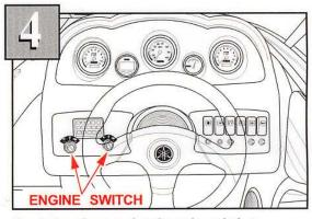
To start engine turn key in main switch to "START." Release key when engine starts.
