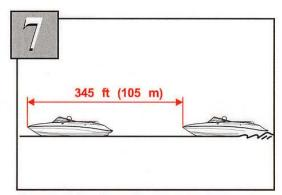
To stop: return the throttle to idle and coast to a stop. There are no brakes on a sport boat. Stopping distance from full speed is approximately 345 feet. You have no steering control with the engine stopped. Do not shift into Reverse at planing speeds. Use Reverse only for low speed maneuvering.
