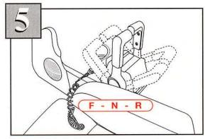
Select Forward or Reverse, then accelerate by gradually pushing throttle lever in the desired direction.
