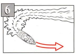
Turn the steering wheel in the direction you wish to travel while applying throttle. YOU NEED THROTTLE TO STEER.
