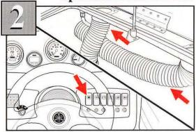
Operate blower for at least 4 minutes and check engine compartment bilge for gasoline vapors before starting engine. Do not start the engine if there is a fuel leak or loose electrical connection.
