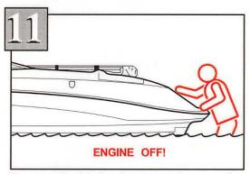
Do not apply throttle when anyone is at rear of boat - turn engines off while boarding from the rear, using the swim platform, or when swimming behind the boat. Water and/ or debris exiting the jet thrust nozzles can cause severe injury, including severe internal injuries if water is forced into body cavities (rectum and vagina).
