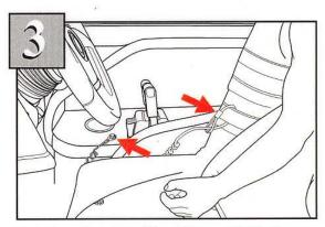
Attach engine shut-off cord to your PFD, then insert cord clip on engine shut-off switch. Failure to attach the lanyard could result in a runaway boat if operator is ejected. The engine cannot be started unless the clip is installed.
